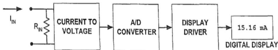
Figure 14.5: Block Diagram of Electronic Ammeter with a Digital Display Readout
