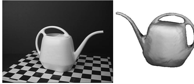
FIGURE 5.3. The picture on the right shows the reconstructed surface from multiple images on the left.
