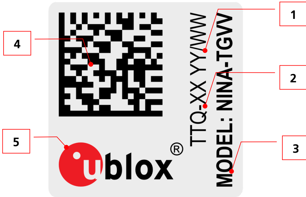
Figure 10: Location of product type number on the NINA-W1 series module label
