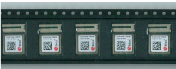
Figure 7: Orientation of NINA-W132 module on tape
